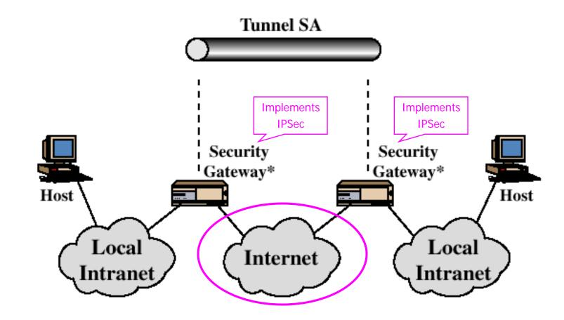
IPSec protects communication on the insecure part of the network
